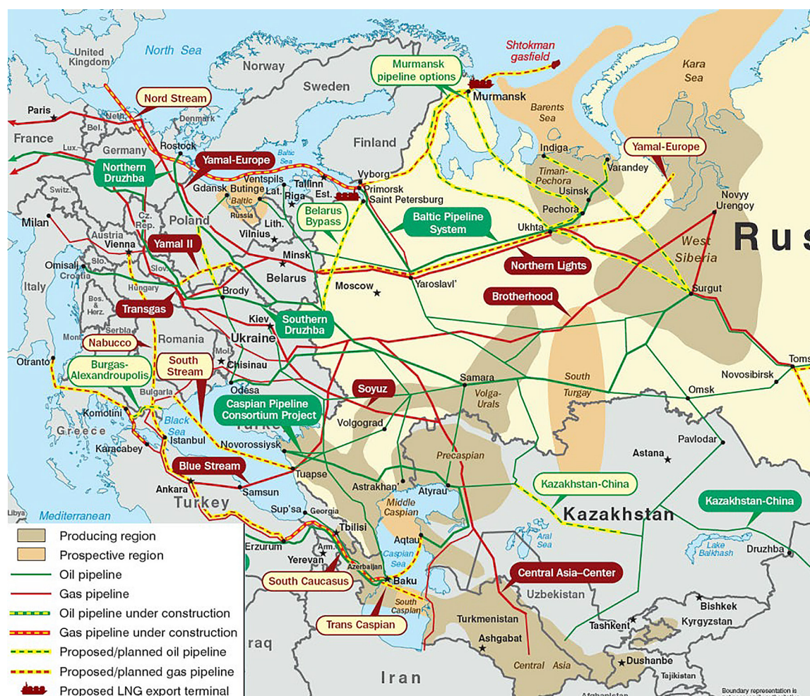
Figure 1. Map of existing and planned oil and gas pipelines across Eurasia
